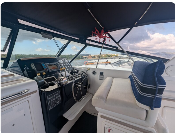
Tiara 4100 Open helm station
